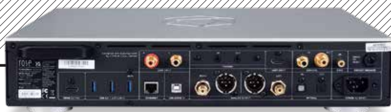
ABOVE: Wired and wireless (via USB dongle) Ethernet inputs are joined by coaxial (to 384kHz/DSD128 DoP), optical (to 192kHz/DSD64 DoP), HDMI eARC and USB-B (to 768kHz/DSD512), plus two USB-A ports for external media (an internal bay accommodates users' own SSD/HDD hardware). RCA line ins are joined by RCA/XLR line outs, HDMI (4K video), USB-A 3.0 plus coax/opt digital outs, and 12V trigger ports
